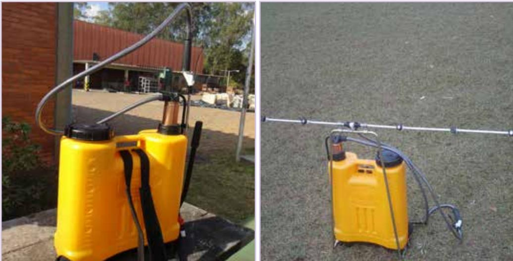
A single nozzle sprayer and multiple nozzle sprayer: Photo by KENDAT
