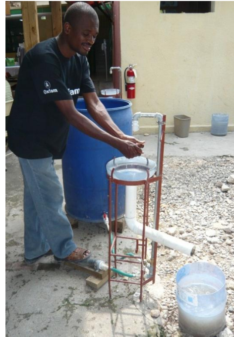
Oxfam prototype handwashing device
