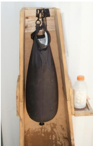
Water bag with push button dispenser on the bottom, liquid soap on the side
