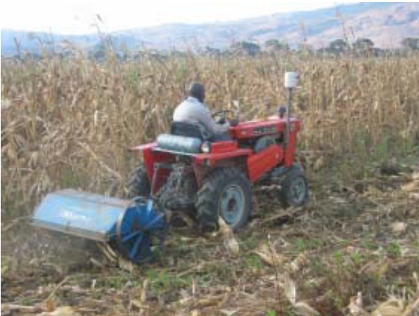
29 Tractor-drawn knife roller for crushing weeds, crop residues and cover crops before planting Josef Kienzle
