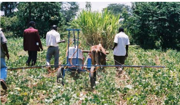
34 Triton draught animal-pulled sprayer with an 80 litre tank and a 5 m boom Brian Sims
