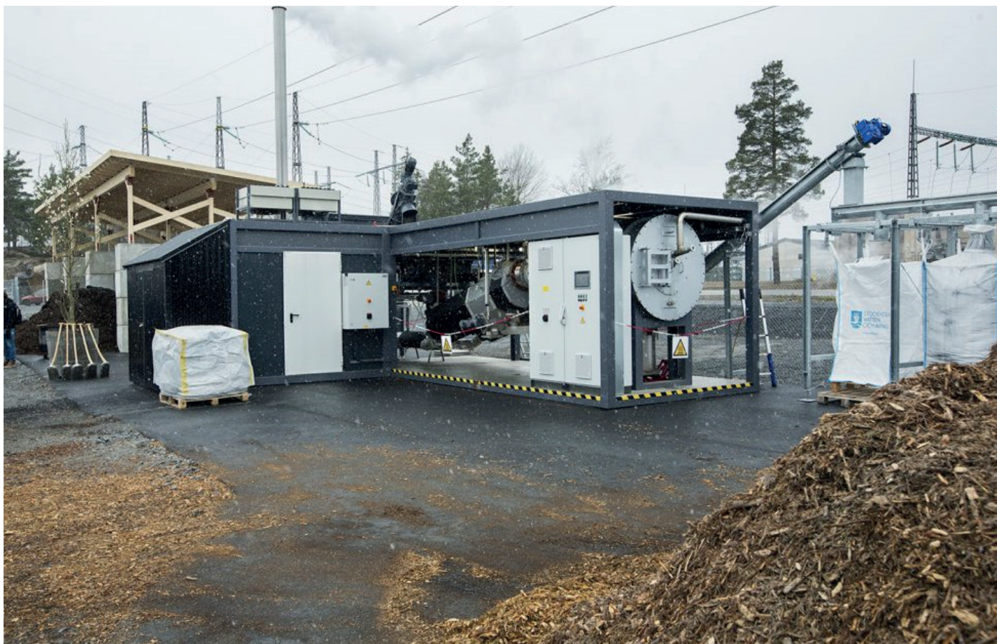
INDUSTRIAL LEVEL combustion chamber for household heating and biochar production.
