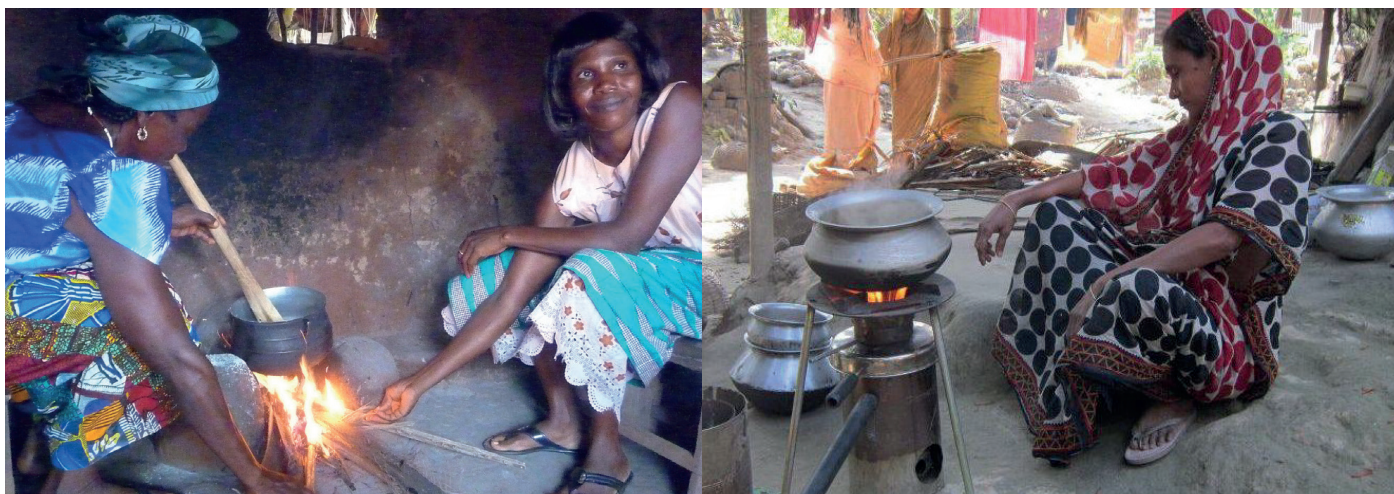
LEFT: popular three-stone technique of household cooking, often performed in black kitchens with poor ventilation and RIGHT: improved rocket stove design with a biochar chamber, saving fuel and effectively cooking without the creation of irritating smoke.
