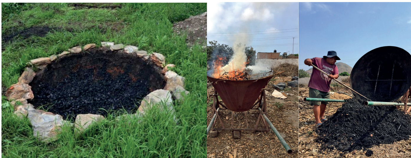
MAKING OF BIOCHAR left: in a conic shaped pit and right: in a metal mobile retort
